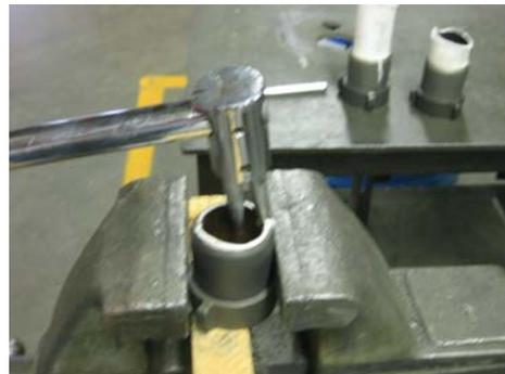
If the hose has a thin wall, the points on the 109 Tool may be too big to get started between the coupling and the ring. In that case, drive the point of a center punch in first to provide a large enough gap for the 109's point.
